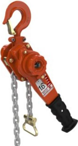
The Hackett L5 QP lever hoist incorporates the four pawl mechanical engagement functionality. The unique and patented pawl design enhances the capabilities of the hoist allowing all four pawls to engage with the ratchet gear in an offset configuration allowing finer adjustment and tensioning capability while maintaining pawl/ratchet engagement. This improves the hoists:
