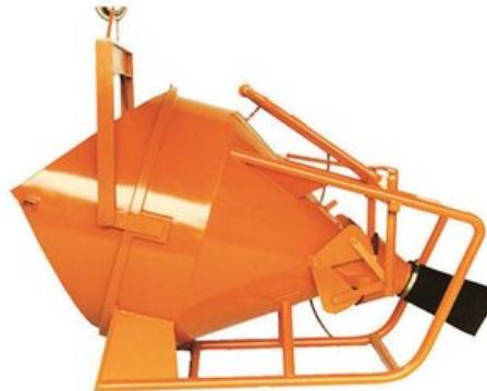
With a range of sizes available, Concrete Column Skips are used for pouring concrete, especially in formwork or columns where access could prove to be difficult.
