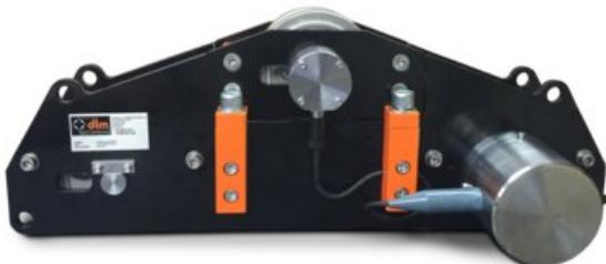
The DLM Standard Running Line Monitor measures the tension on a rope passing through its three wheels. Typically used in cable laying and winch operations to measure and record line tension the robust design has become an industry standard. The monitor can be supplied as a separate item for integration with customers existing PLC's or with a DLM digital display/HMI touch screen display.
