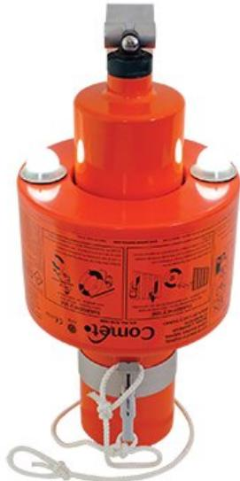
SOLAS requires one of these markers to be mounted on each bridge wing attached to a 4kg lifebuoy. Mounted in its steel bracket on each bridge wing attached to a lifebuoy. Signal can be mounted up to 56m above sea level. (SOLAS only requires>30m). Produces dense orange smoke for 15 minutes and 2 LED lights burn at 2 candela for 15 hours minimum. Signals location of a man overboard by day or night.
